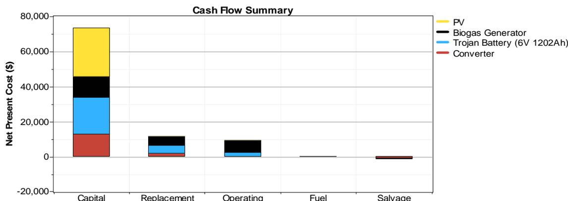
Fig. 9. Cost summary of the PV/biogas power system.
