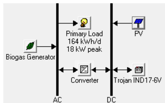
Fig. 6. Schematic of system configuration.
