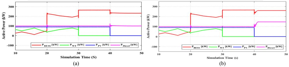
Fig. 6. Active power profile in Geocha microgrid: (a) CVCF only; (b) Proposed.
