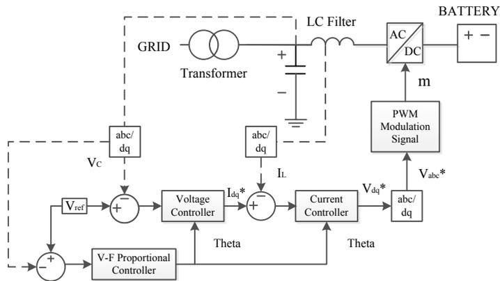
Fig. 2. Grid-forming BESS configuration with control algorithm.
