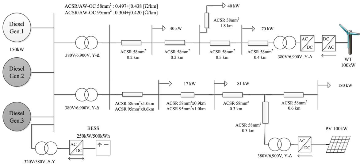
Fig. 1. Geocha Island microgrid system configuration.
