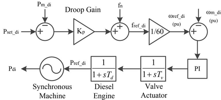
Fig. 4. Control structure for active power of a diesel generator.
