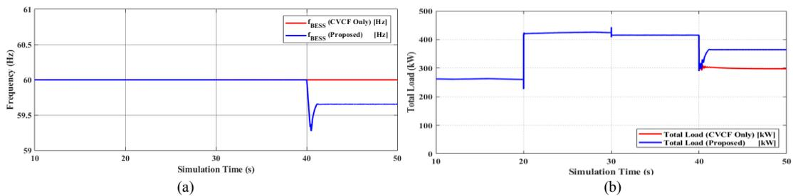
Fig. 8. Comparison of system profile in Geocha microgrid: (a) System frequency; (b) Total load.
