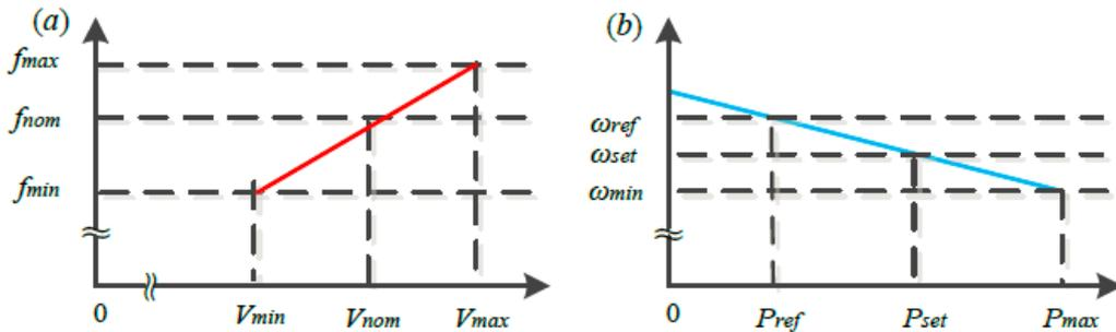
Fig. 5. (a) VFPC scheme in the BESS; (b) conventional droop characteristic.
