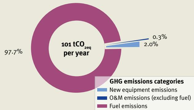
**Figure 3:** GHG emissions breakdown of a 13 kW diesel-based mini grid for institutional use in Nyabiheke refugee camp, Rwanda, powering basic services for 13,000 refugees.
